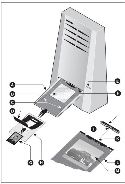
Figure 6: Operating the Flextight 646 scanner
